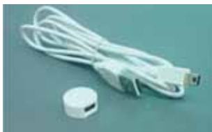
Exterior EHF oscillator and cable
